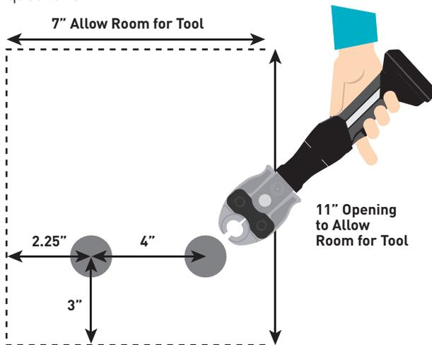
**15. What can I use to make inserting larger copper tubes into the Zoomlock fittings easier?**
